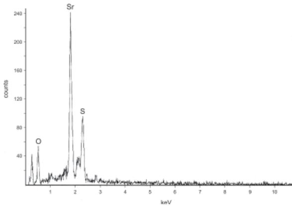
Fig. 7. X-ray energy dispersive spectroscopy (EDS) spectrum of *Dorataspis micropora* Haeckel. Spectrum obtained with X-ray spectrometer examined at 15 kV for 100 live second. Data indicates the existence of strontium, sulfur, and oxygen within the skeleton.
