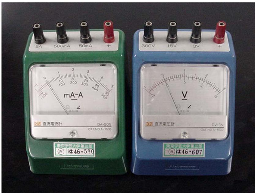
Fig. 1 An ammeter and a voltmeter used in elementary school and junior high school in Japan.
